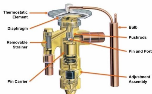
Fig 20: Thermostatic Expansion Valve (TXV) (left)
