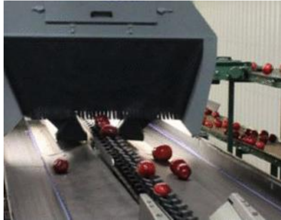
Fig. 1: Optical Grader Capturing Image
